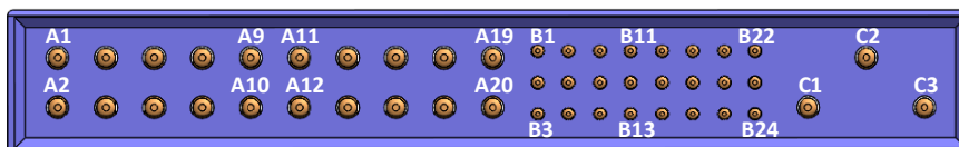
Figure 1-7: IN/OUTPUT CONNECTOR POSITRONIC P/N: PCIH47M400A1/AA
